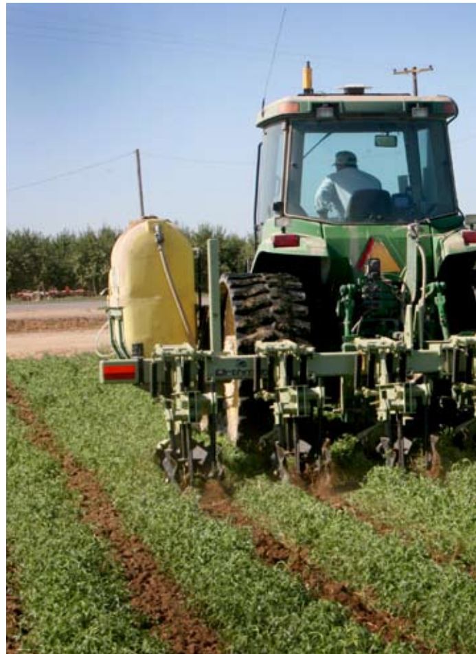
Figure 3. Orthman 1-tRIPr strip tilling alfalfa prior to corn planting, Helm, California, July 9, 2005. Photo: J. P. Mitchell.
