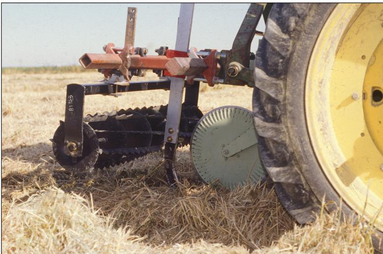
**Figure 3.** Basic components of early prototype strip-till implement used in California, including residue-cutting coulter, subsoiler shank, and clod-busting rolling basket, Five Points, California, 1996. Photo: Jeff Mitchell.
