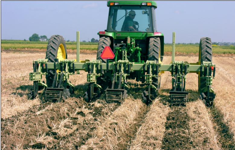
**Figure 4.** Ground-driven modified Orthman 1-tRIPr strip-tiller implement tilling in cover crop in center of tomato beds and sweeping out furrows for irrigation, Davis, California, 2006. Photo: Dennis Bryant.
