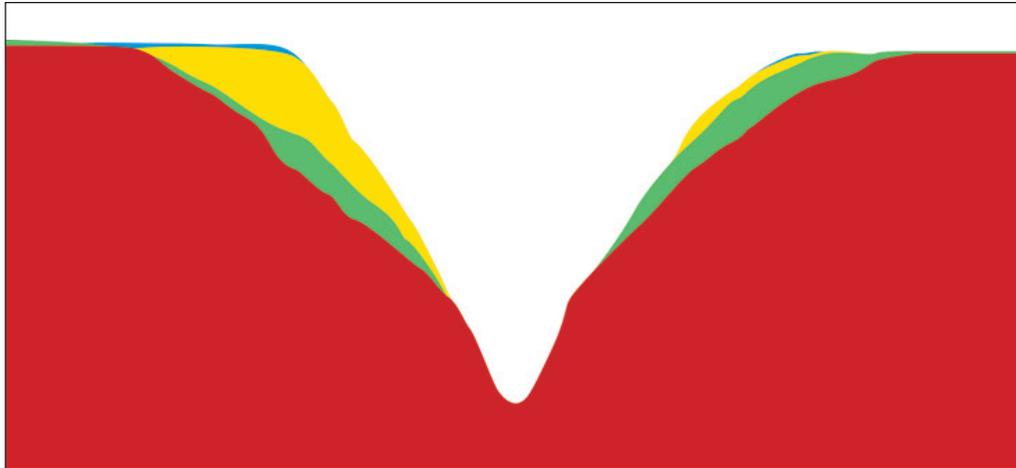
**Figure 8.** Model of soil cross-section showing extent of soil-loosening when strip-tillage is done when soil is wet (yellow) or dry (green). Red indicates soil that is not affected by the strip-tillage shank. Courtesy Randy Raper and Francisco Arriago, USDA ARS Soil Dynamics Laboratory, Auburn, Alabama, 2007.
