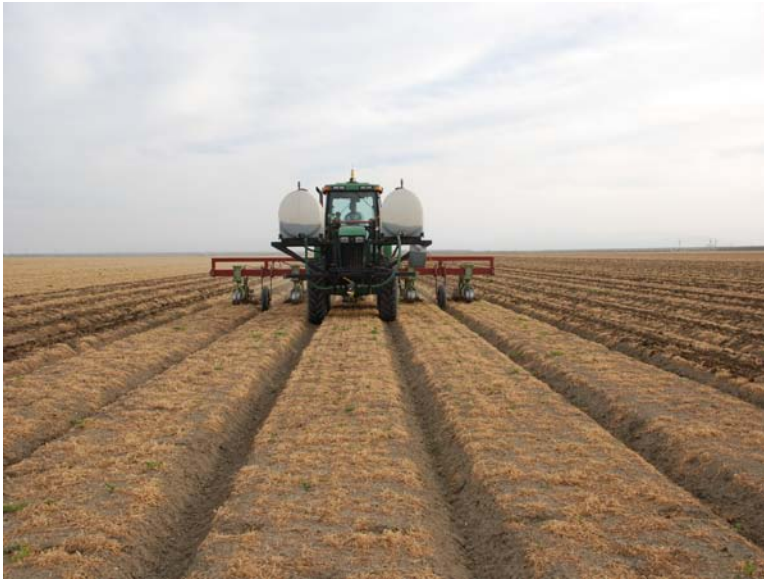
Photo 7. Modified Orthman 1-tRiPr 5-row strip-till implement tilling in cover crop residue and incorporating pre-plant herbicide prior to tomato transplanting at Sano Farm, Firebaugh, CA, 2009
