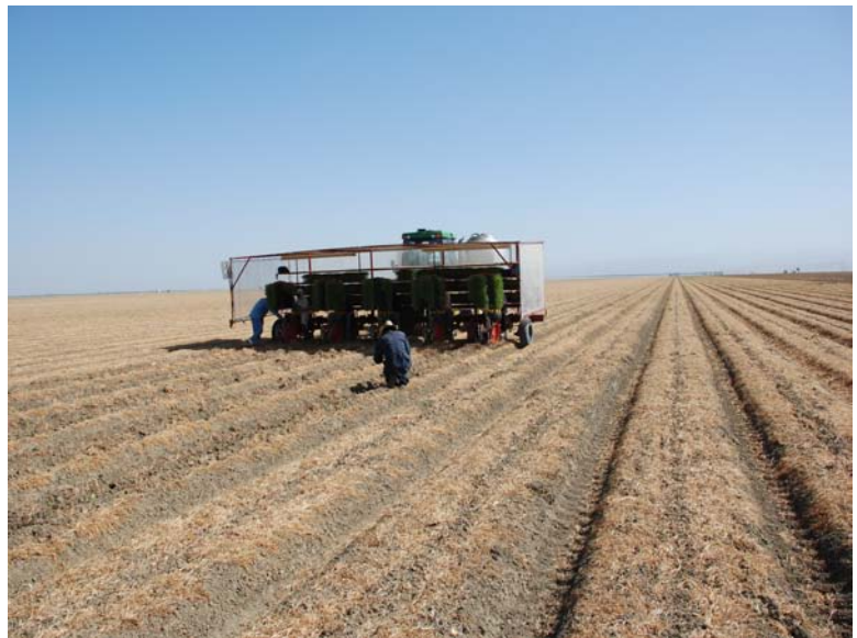
Photo 11. Conventional 5-row tomato Checcli Magli® (Hahn Tractor, Stockton, CA) transplanter that is used to establish tomato seedlings in cover crop residues at Sano Farm, Firebaugh, CA 2009
