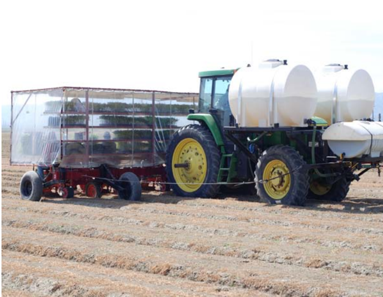
Photo 12. Conventional 5-row tomato transplanter that is used at Sano Farm, Firebaugh, CA, 2009
