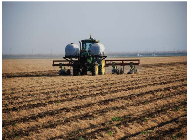
Photo 8. Ground-driven strip-tiller used to prepare bed centers prior to transplanting, Sano Farm, Firebaugh, CA, 2009
