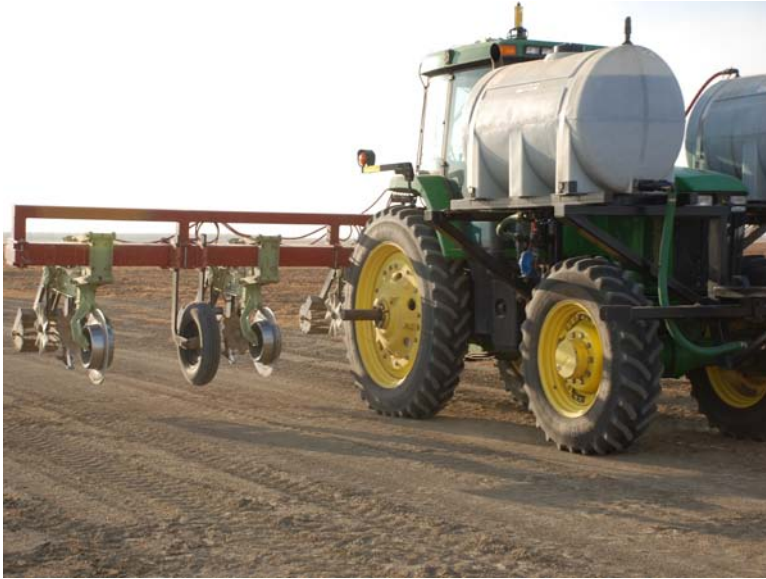
Photo 9. Close-up view of modified Orthman 1-tRiPr strip-till row units on Sano Farm strip-tiller showing residue-cutting depth wheel and coulters, subsoiling shank, wavy coulters, and clod-busting rolling baskets.
